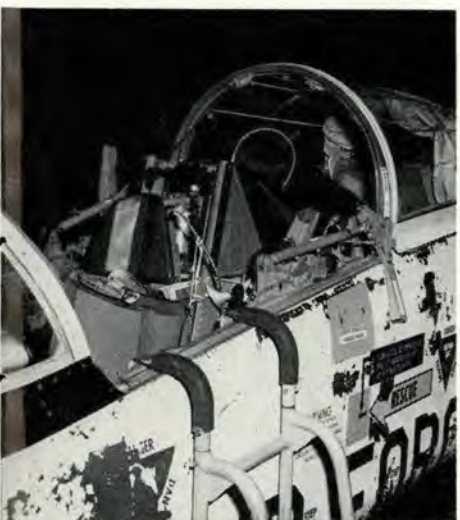
Above, wheel failure and, below, materiel failure due to improper adjustment resulted in loss of the T-38 canopy.
