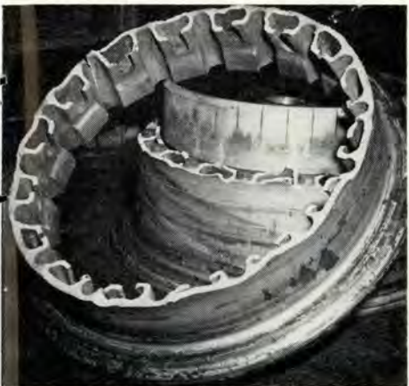
Above, wheel failure and, below, materiel failure due to improper adjustment resulted in loss of the T-38 canopy.
